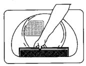
The lint filter should be removed at the end of each drying cycle for cleaning. It should be lifted straight up until it clears the door opening. Remove the lint with your hands. Be sure the lint filter is properly replaced.
